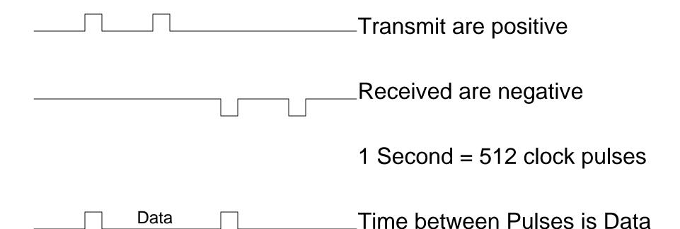
Clock Pulses between leading edges = (Code x 16) + 8
